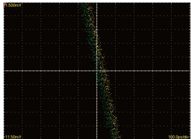
Figure 5. Using SMC TClk synchronization, multiple NI PXIe-5442 modules can achieve <20 ps channel-to-channel skew.
