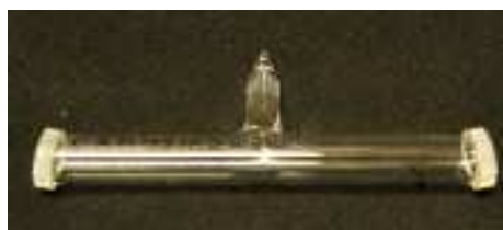
Optical Cell featuring wedged and angled window design
