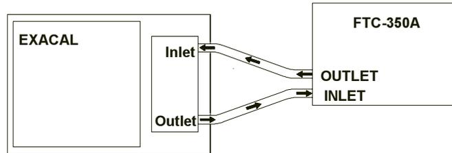
Connect the FTC-350A INLET to the outlet of the EXACAL circulating pump.
