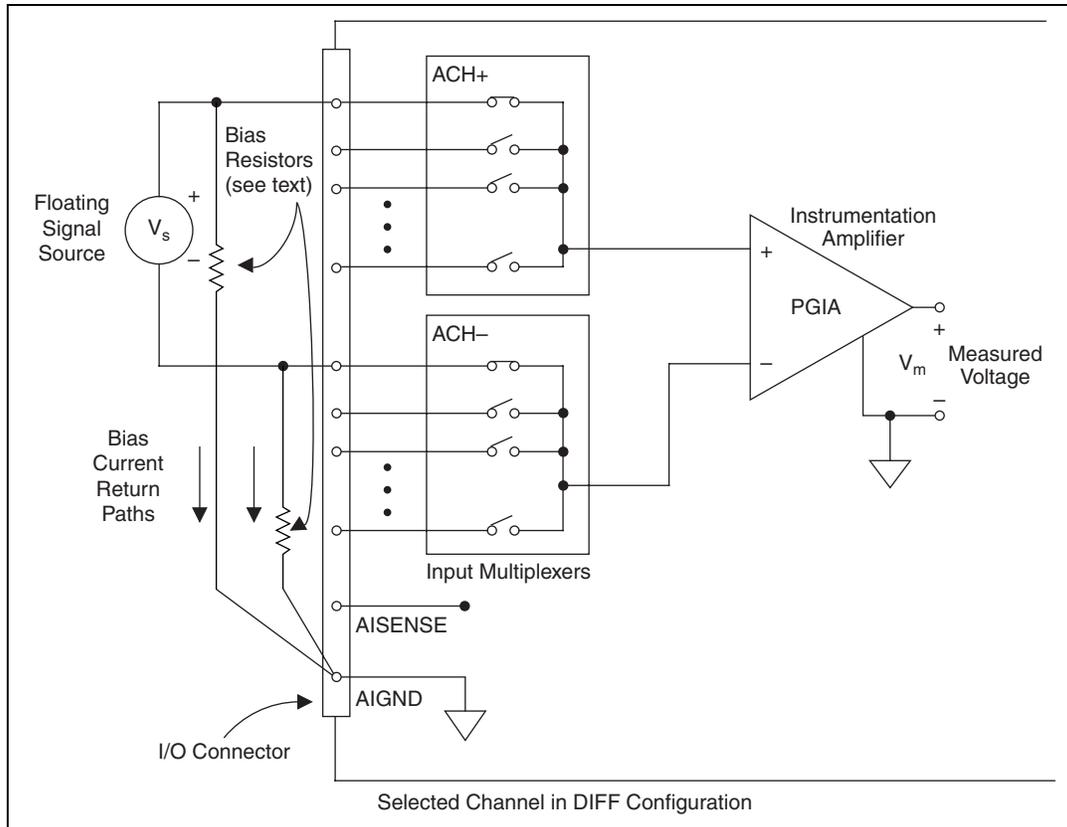
**Figure 4-5.** Differential Input Connections for Nonreferenced Signals
