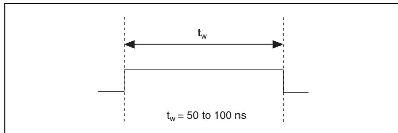
**Figure 4-14.** TRIG1 Output Signal Timing
