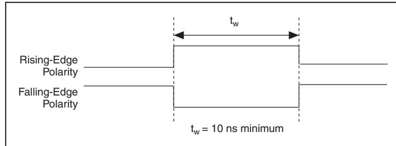
**Figure 4-33.** GPCTR1\_GATE Signal Timing in Edge-Detection Mode
