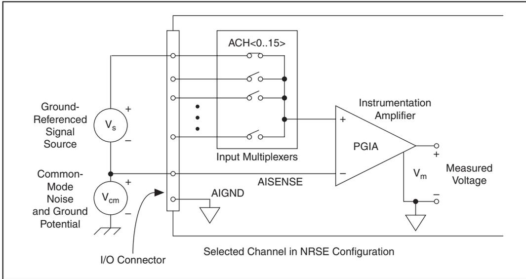
Figure 4-7. Single-Ended Input Connections for Ground-Referenced Signals
