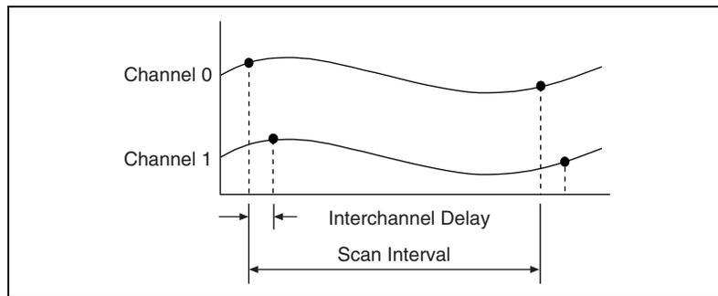
**Figure C-2.** Scan Interval
