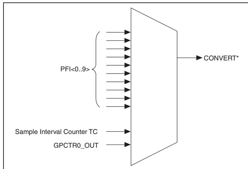
**Figure 3-2.** CONVERT\* Signal Routing
