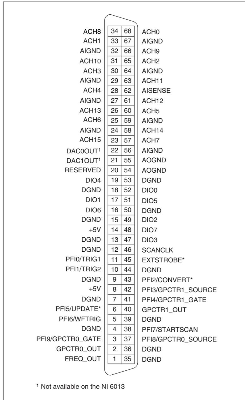
Figure B-1. 68-Pin Connector Pin Assignments
