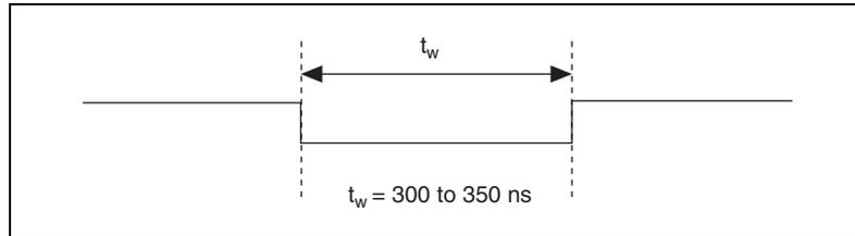
**Figure 4-27.** UPDATE\* Output Signal Timing
