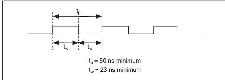
**Figure 4-32.** GPCTR1\_SOURCE Signal Timing
