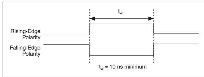
**Figure 4-30.** GPCTRO\_GATE Signal Timing in Edge-Detection Mode
