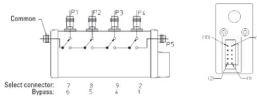
**Table 3. Keysight 8769M with switch profile and connector pin assignments**
