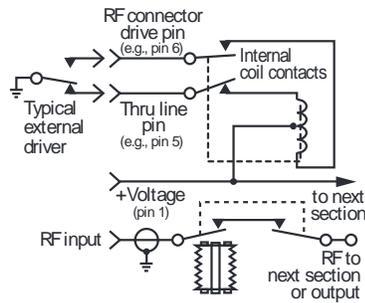
Figure 2: Port electrical diagram
