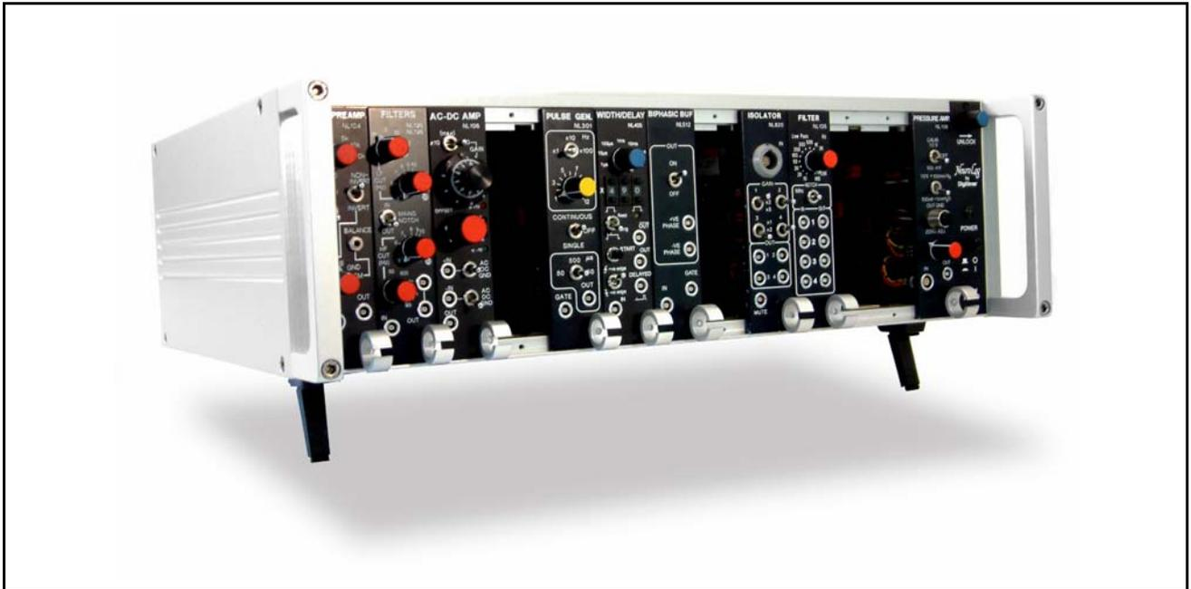
The NL900 NeuroLog module frame and power supply are housed in a fully finished, enclosed case. The case has carrying handles and is supplied with bolt-on rack mounting hardware so that it can be located either in the rack or on the bench top. The base is fitted with rubberised feet and the front pair may be extended so as to raise the front of the unit. These are easily removed, if required, for rack-mounting.
