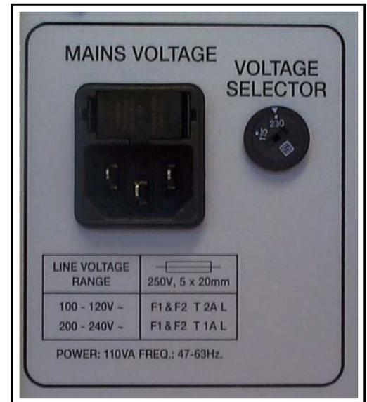
Changing the mains voltage will also require you to change the two fuses in the mains inlet. They must be “5 x 20 mm” in size and the value and speed shown here.
