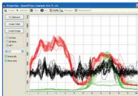
*This figure shows a measurement of fluorescence intensity with the help of a line profile. The profile clearly shows the concentration of the histone H2B protein, which has been linked to the fluorescent protein DsRed.*
