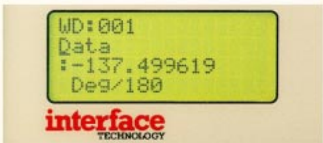
Word number one from the above example is programmed with a data value of -137.499619 degrees of angle. Up to 511 more data values may be entered.
