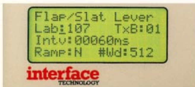
Transmit menu shows one of 16 labels defined as label 107 with a 60 ms update rate of 512 words of data.
