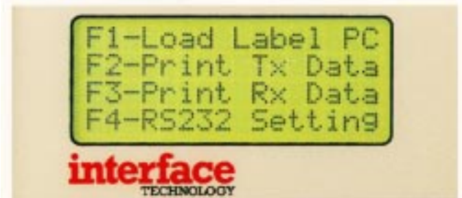
The RS-232 port may be used to upload new label definitions, save system configurations, load system configurations, or print data to a printer or host computer.
