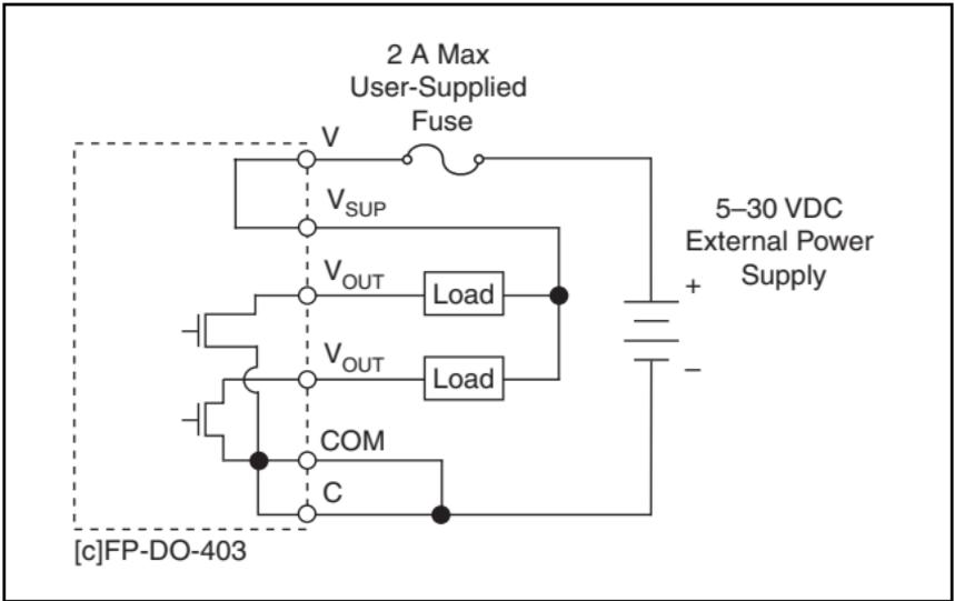
**Figure 3.** Wiring for Low-Current Applications
