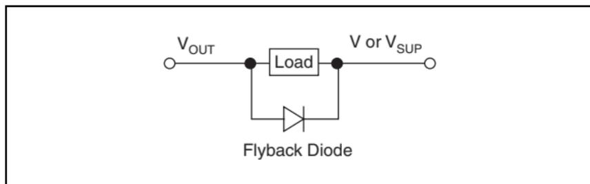
**Figure 5.** Connection to Inductive Load with Flyback Diode
