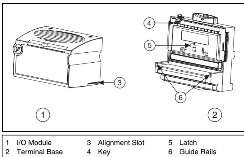
**Figure 1.** Installing the FP-DO-403
