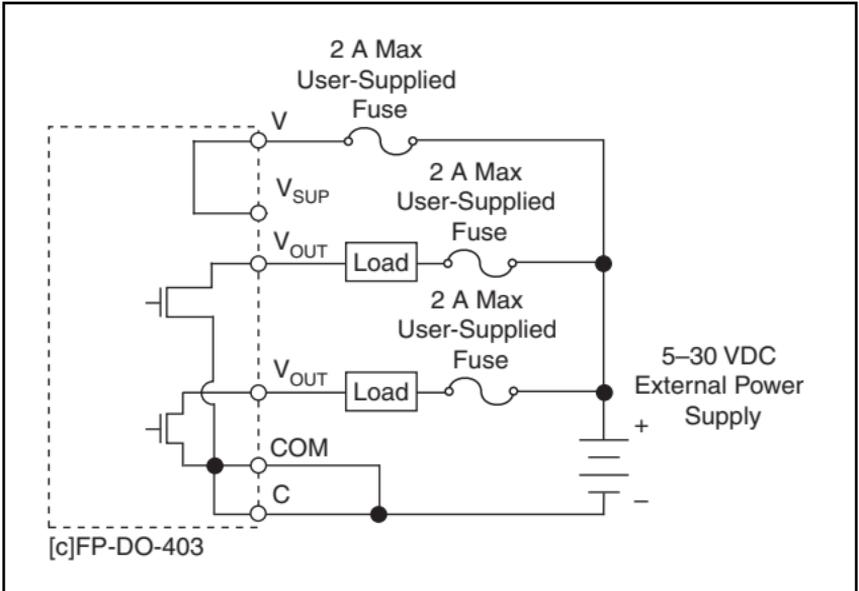
**Figure 4.** Wiring for High-Current Applications
