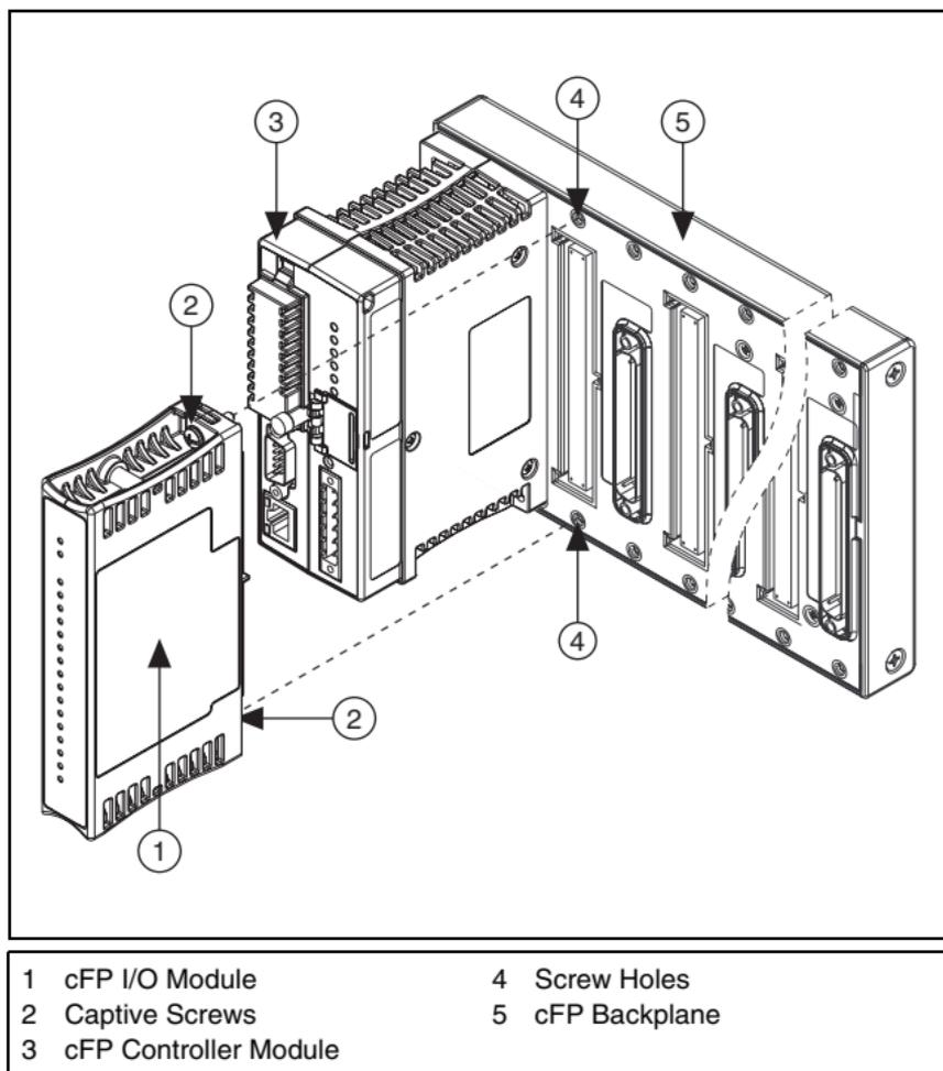
**Figure 2.** Installing the cFP-DO-403
