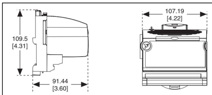
**Figure 6.** FP-DO-403 Mechanical Dimensions
