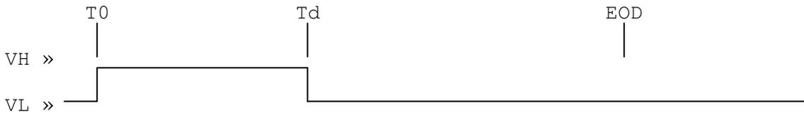
MODE 5: T0/delay - Same as mode 4, but output polarity is inverted.
