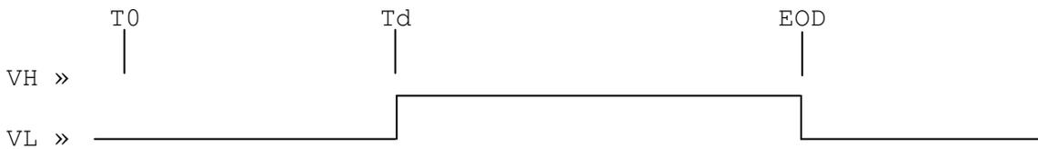
MODE 1: DELAY - Negative edge at programmed delay time. Level is maintained until EOD.
