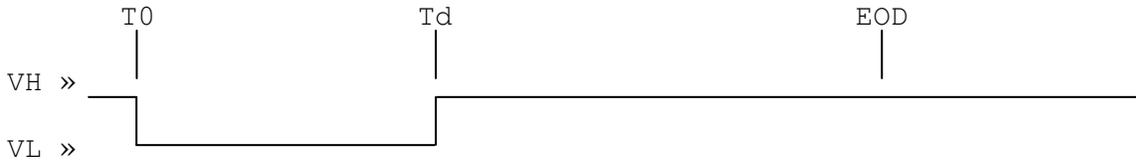
MODE 6: OR-ALL Logical OR of all timing channels (1...4 or 1...6); output is active high. Used primarily when all channels are in ONESHOT mode, as shown here:
