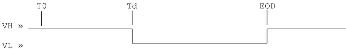
MODE 2: WIDTH + Two channels are paired (1/2, 3/4, or 5/6). The output goes high when the ODD channel delay is reached, and returns low when the EVEN channel times out. For Channels 1 and 2, this signal is  $OUT = (T1 * !T2)$ .
