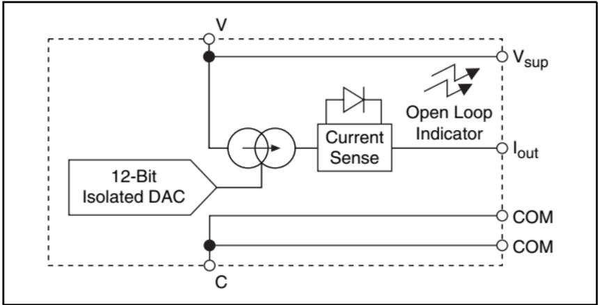
**Figure 3.** [c]FP-AO-200 Current Output Circuit
