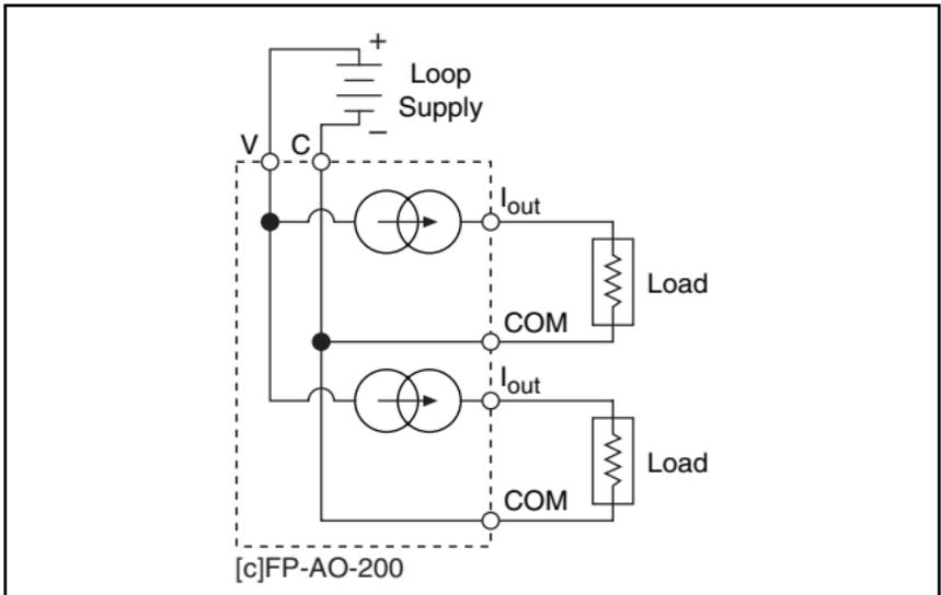
**Figure 4.** Connecting to Two Channels
