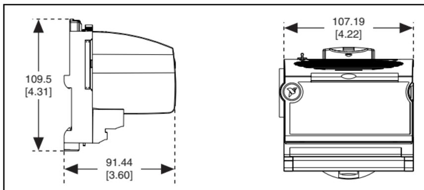
Figure 7. FP-AO-200 Mechanical Dimensions
