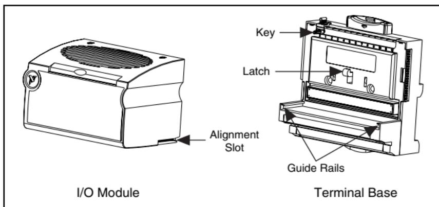
**Figure 1.** Installing the FP-AO-200
