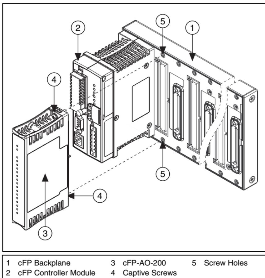
**Figure 2.** Installing the cFP-AO-200
