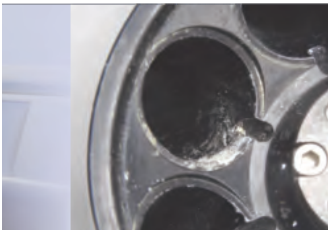
Heavy corrosion can result in premature rotor failure.
