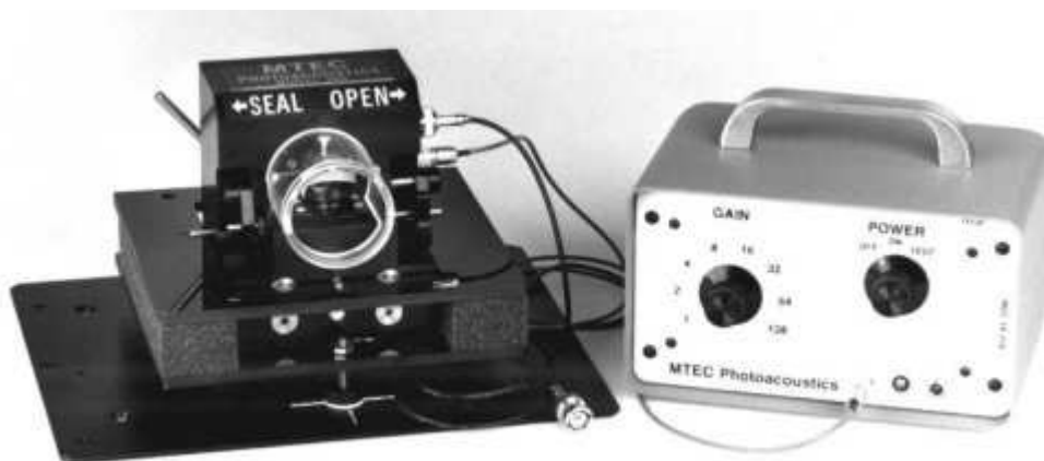
Fig. 3. MTEC Model 200 photoacoustic detector mounted on a Nicolet sample compartment baseplate.
