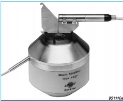
Fig. 1 Mouth Simulator shown with pressure Microphone Type 4134 in jig for calibration according to CCITT P.51. For calibration to IEEE 269, free-field Microphone Type 4133 can be fitted ( 0^\circ incidence)
