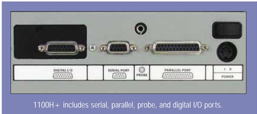
1100H+ includes serial, parallel, probe, and digital I/O ports.
