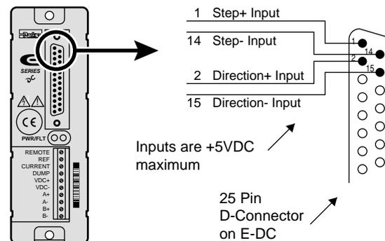
*Test Configuration – E-DC Step and Direction Inputs*
