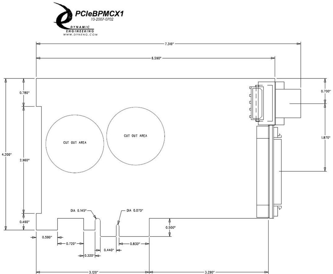
Previous revision outline. Current boards have relocated zero slot fans to allow both fans to be used and stay within the height envelope allowed by PMC specification.
