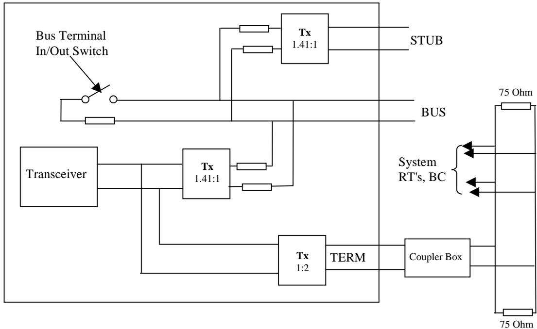
**Figure 13-4 Replacement of RT/BC (but not the coupler box) in an existing system**
