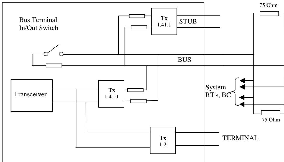
**Figure 13-5 Replacement of RT/BC and coupler box in an existing system**
