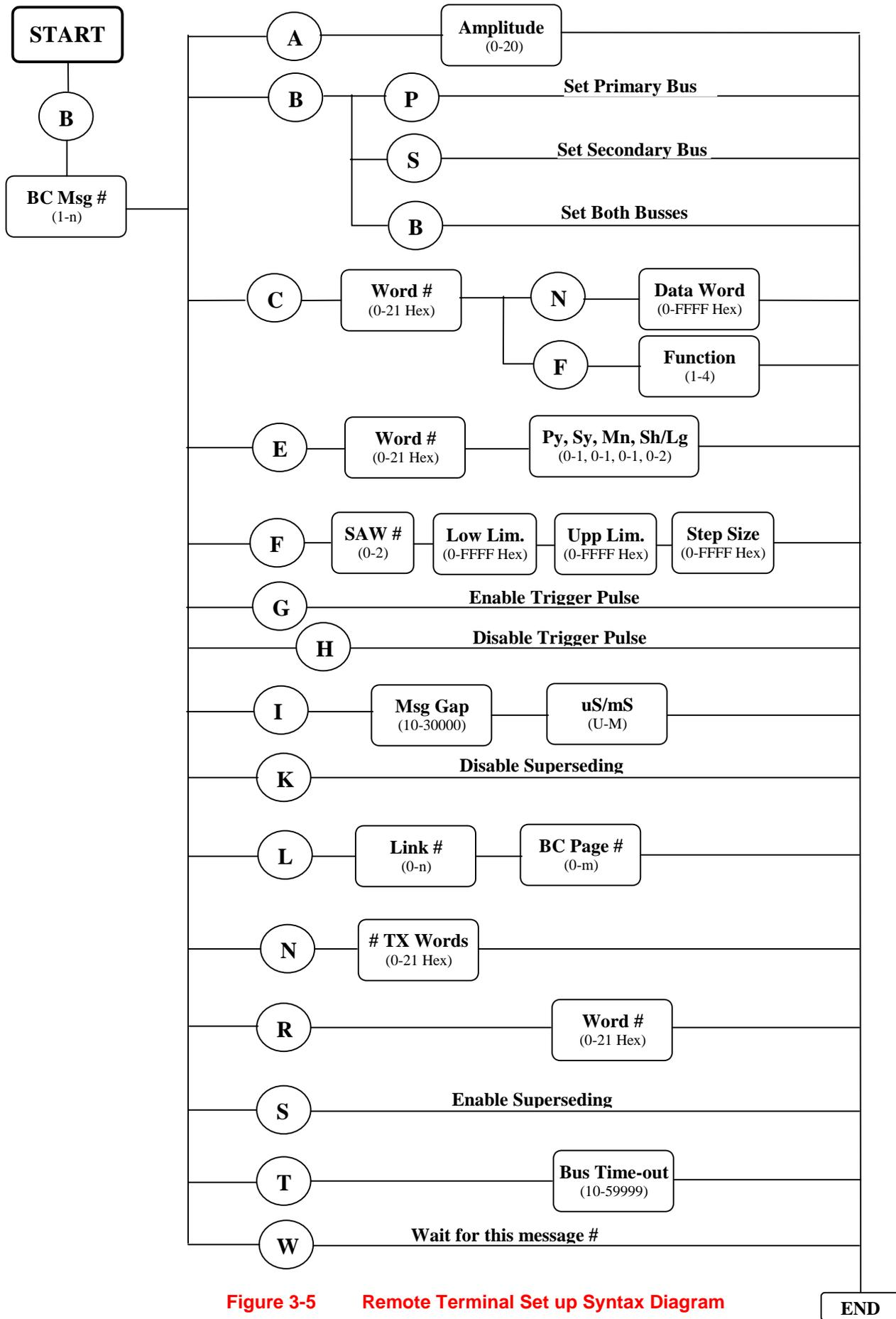
**Figure 3-5 Remote Terminal Set up Syntax Diagram**
