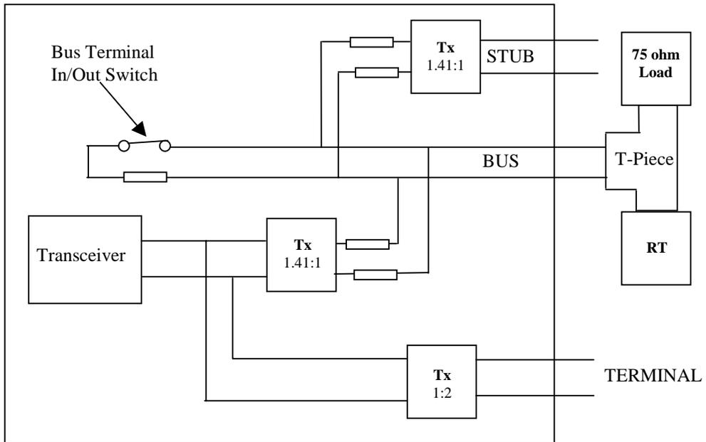
**Figure 13-3 Bench testing Direct Coupled Stub on 1553 device**
