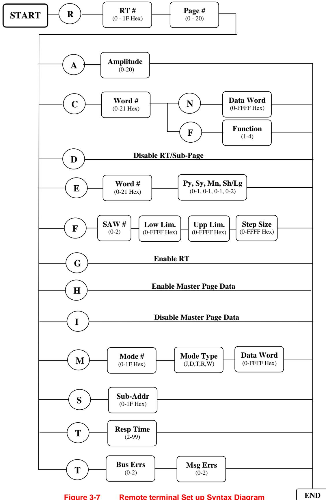
**Figure 3-7 Remote terminal Set up Syntax Diagram**
