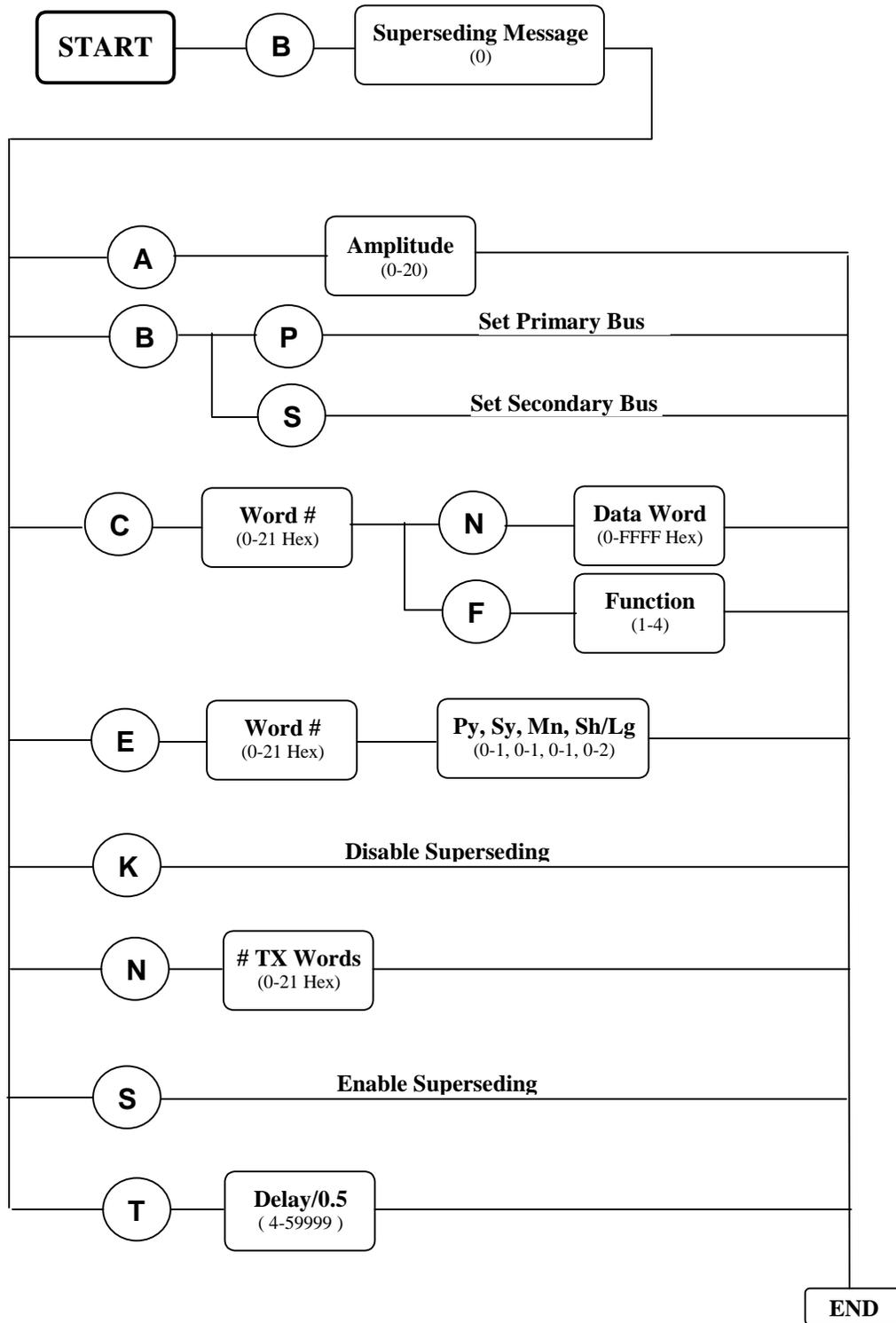
**Figure 3-6 Superseding Command Set-up Syntax Diagram**
