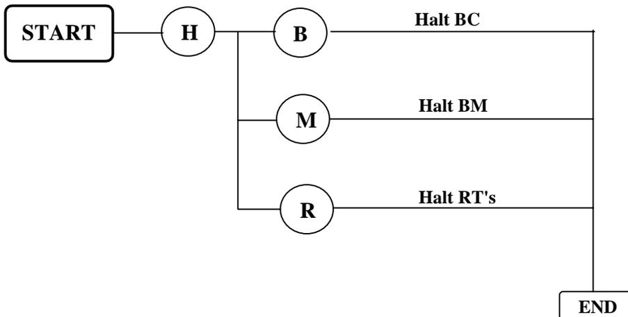
Figure 3-10 Halt BC, RT, BM Syntax Diagram
