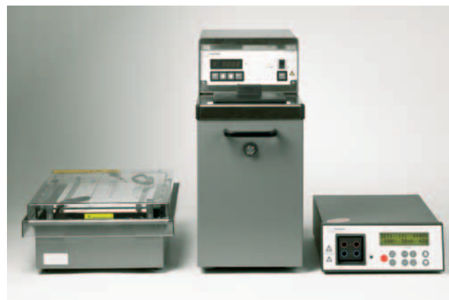
Fig 1. Main components of Multiphor II Electrophoresis System: Multiphor Electrophoresis Unit, MultiTemp III Thermostatic Circulator and EPS 3501 XL Power Supply.
