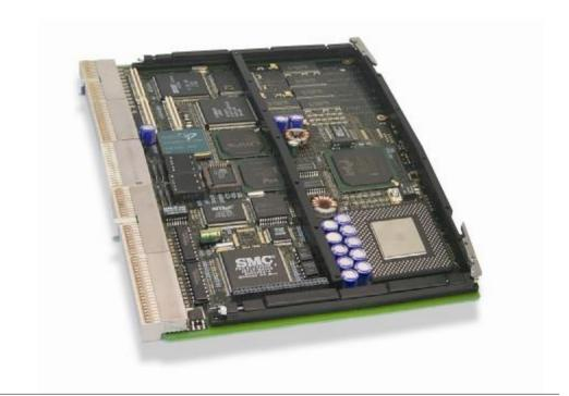
**CR7** is a CompactPCI<sup>®</sup> all-in-one 6U single board computer designed to meet the needs of embedded application developers addressing markets like industrial automation, medical, scientific, imaging, telecommunication, military and aerospace.
