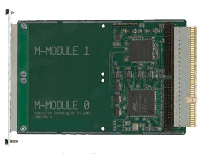
The i3002 provides a high-performance CompactPCI bus gateway to the M-module interface. The i3002 has a 3U form factor. Two M-modules can be mounted on the i3002. The M-module interface of the i3002 complies with the M-module specification. The M-module interface feature A8, A24, D16 and D32 access types.
