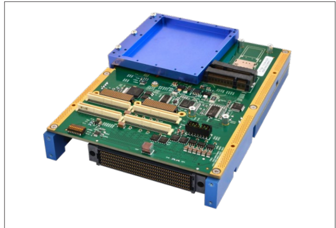
ACEX-4610 carrier card bottom view showing PMC/XMC slot
