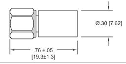
Model Number: **TE400F** 2.4mm Female Connector DC - 40 GHz
