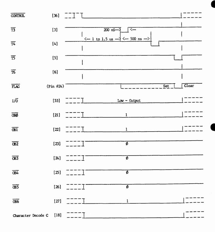
Figure 450-1: Timing Diagram - Output Character C from System Controller
