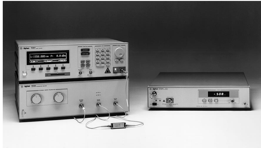
Figure 5. Polarization mode dispersion measurement setup using the Agilent 8509B and Agilent 8168 or Agilent 83424 lightwave sources.
