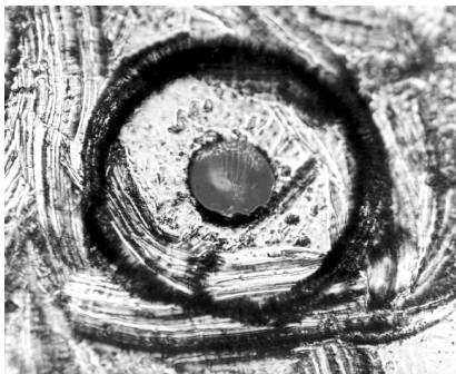
Figure 6-5. A damaged fiber end from using an improper cleaning procedure
