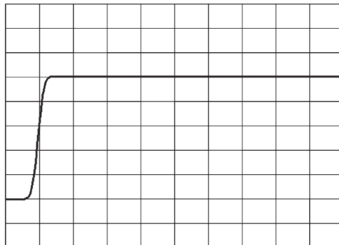
Figure 13 Step response of 4 MHz analog alias filter with 12-tap compensation giving a Gaussian response with 1 MHz 3 dB bandwidth. Horizontal scale is 1 \mu\text{s}/\text{div}
