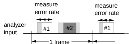
Figure 8: Individual cell segments can be measured, i.e. only payload
