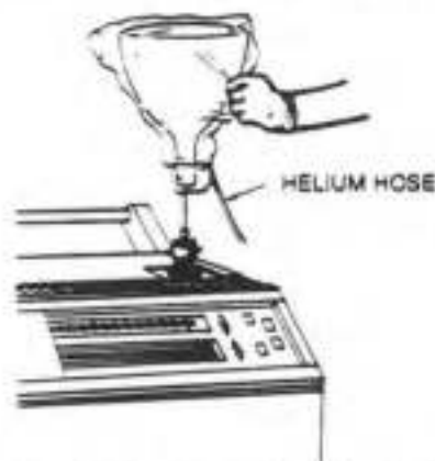
Figure 1-6. CRT evacuated and tested with a conventional automatic leak detector. The CRT is hooded to insure the integrity of the entire tube.
