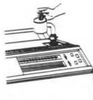
Figure 1-10. A Bourdon gauge, pre-bombed with helium, under test.
