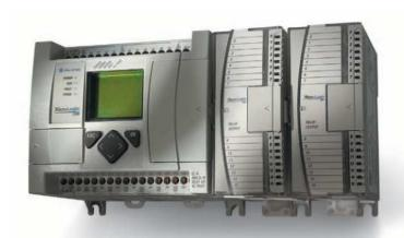
With online editing and a built-in 10/100 Mbps EtherNet/IP port for peer-to-peer messaging, the MicroLogix 1100 controller adds greater connectivity and application coverage to the MicroLogix family. The next generation controller's built-in LCD screen displays controller status, I/O status, and simple operator messages; enables bit and integer manipulation; and offers digital trim pot functionality.
