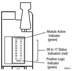
The front panel of your module contains 18 status indicators. The green top indicator is labeled "ACTIVE." This indicator is on when the fuse is good. The green bottom indicator, when on, indicates you selected high-true logic. When off, it indicates you selected low-true logic.
