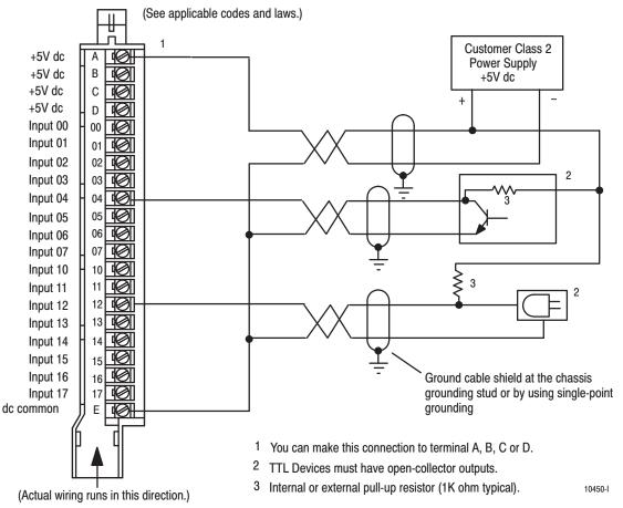
Do not exceed the specified isolation voltage when using multiple power sources.
