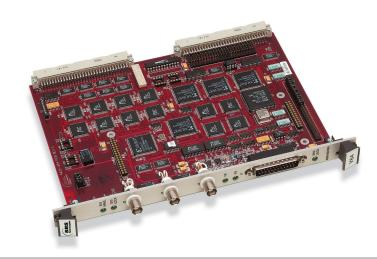
**4422-V64** is a complete, system level telemetry module for the VME bus. The module supports all of the functions required for telemetry data acquisition for input data streams at rates up to 20 Mbps.
