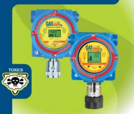
The Series 4600 Gas<sup>PLUS</sup> is a toxic gas and oxygen transmitter designed for single and multi-point monitoring applications where ruggedness, flexibility, and ease of maintenance are critical. The basic Series 4600 transmitter is a two-wire device providing a 4-20 mA output. For additional output flexibility, Series 4600 MB transmitters offer RS-485/232 MODBUS® RTU output and relay contacts in a multiwire configuration.
