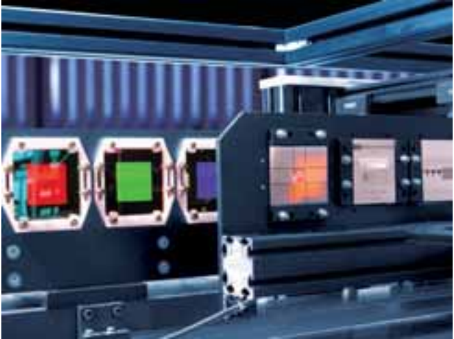
Cameras are measured by the CTT+ according to the EMVA 1288 standard
