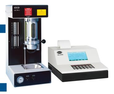
The HIAC 8011 liquid particle counting system provides immediate particle concentration data for low and high viscosity fluids. Composed of a light obscuration or dual-mode sensor, the HIAC 8011 system pressurizes fluid in a HIAC ABS-2 (Automatic Bottle Sampler) for precise volumetric sampling of industrial fluids.
