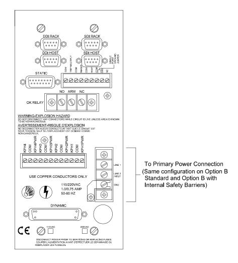
Primary power connections for 3300/12 ac Power Supply (Standard PIM shown)
