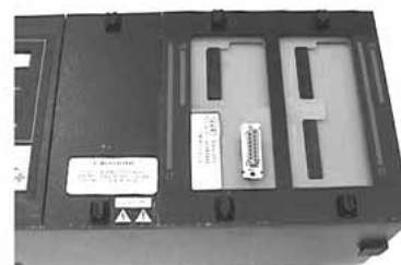
Single-high adapter mounted in scanner position J1.
