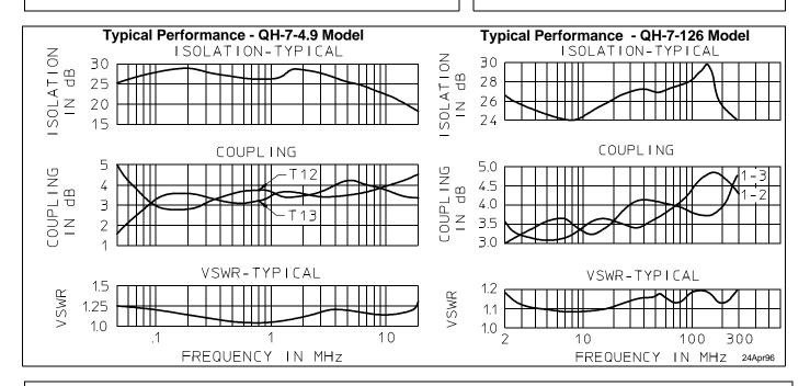
100 kHz to 250 MHz / Multi-Section Lumped Element Designs / BNC & SMA Versions
