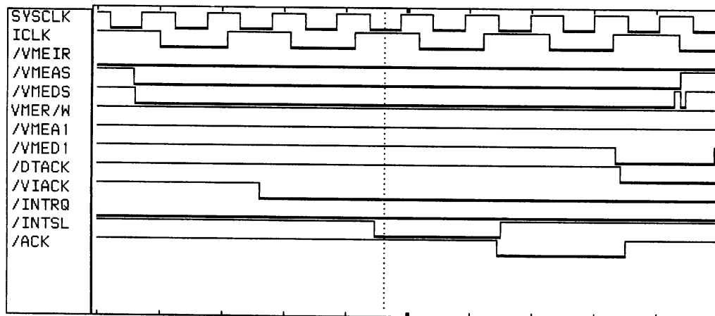
Figure C- 11 IP Module Interrupt Vector Cycle (Snapshot taken at 60 ns/Div)
