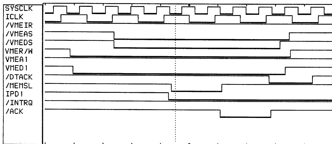
Figure C- 6 Memory Write (Snapshot taken at 70 ns/Div)
