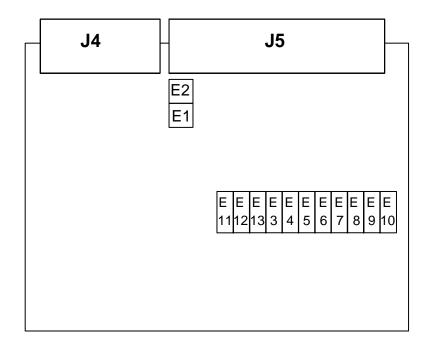
E1 and E2, Factory setting: E1 IN, E2 OUT. Should NOT be modified by user.
