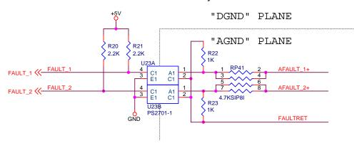
For single ended amplifier fault inputs, typically the AFAULT+ would be the actual signal input from the amplifier and the AFAULT- can be considered the reference.
