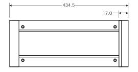
4U standard rackmount chassis shown. 4U extended rackmount chassis differs only in depth (554 mm).
