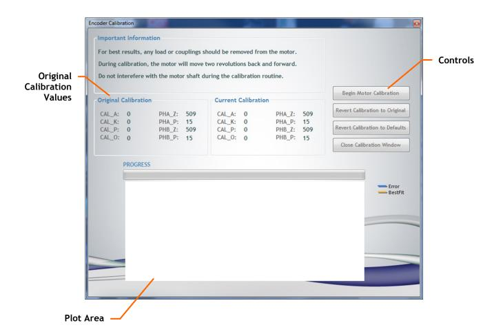
This window shows the original calibration values currently stored in the EvoDrive. You can reset the calibration values to default settings by pressing the Revert Calibration to Defaults button.
