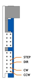
The EvoDrive ST-PCB can be controlled via its digital inputs rather than serial communications. This form of control is useful when interfacing with CNC motion controllers or when implementing complex movement profiles.
