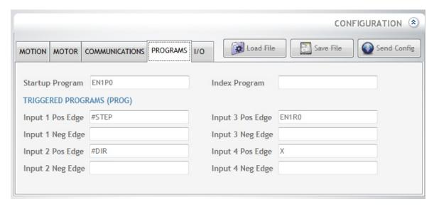
The startup program will ensure the EvoDrive is in a position holding mode immediately after power on.
