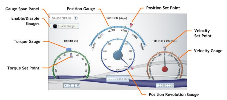
The gauges provide real time feedback for motor torque, position, and velocity. Each gauge has a numerical and a graphical readout which are updated approximately 10 times per second.
