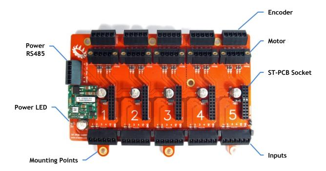
All connectors on the ST-PCB Caddy are 3.81mm pitch pluggable screw terminals (eurostyle). These are a very common type of connector supported by many manufacturers. It allows the flexibility to source specific orientations and termination options. Below are a handful of compatible part numbers:
