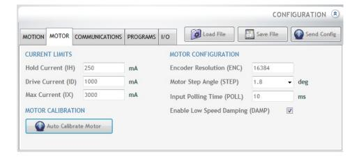
If there is no encoder attached (and configured) on the EvoDrive, then the motor will be calibrated immediately. This will produce a short beep or hiss from the motor, then a prompt will appear to say the calibration is complete.
