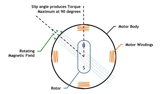
Normally the strength of this magnetic field, which is a function of the current, should be strong enough to overcome any expected acceleration or obstacles. If it is not, then the rotor can't keep up with the field and the motor loses sync.
