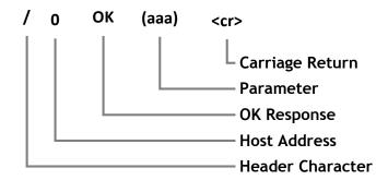
Stackable commands do not return replies individually. On successful completion of a stack of commands, the EvoDrive will return an empty OK response:
