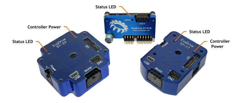
The Status LED is a combination red and blue LED which provides instant status feedback.
