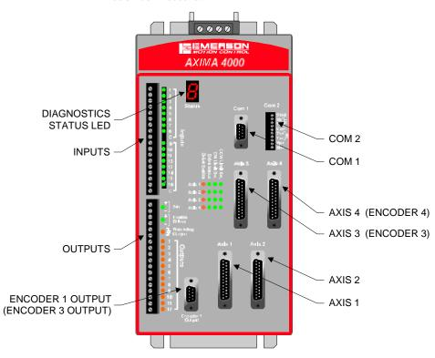
Figure 19 AXIMA 2000/4000 Connectors (4 Axes)
