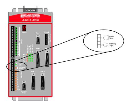
Figure 32 Enable Drives and Watchdog Output Locations on the Front Panel of the AXIMA 2000/4000
