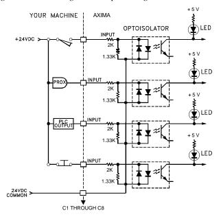
Figure 36 Sourcing Mode Input Diagram
