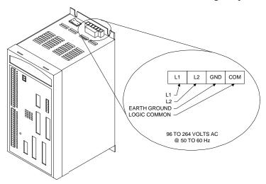
Figure 8 AC Power Connector
