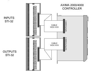
Figure 46 AXIMA 2000/4000 Direct Wiring Option Using STI-32's
