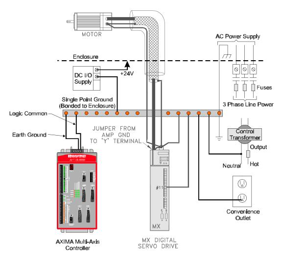
Figure 6 MX Drive and AXIMA System Grounding Diagram
