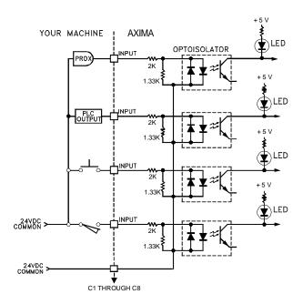
Figure 35 Sinking Mode Input Diagram
