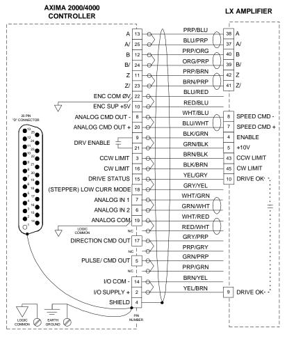
Figure 29 AXIMA 2000/4000 to LX Amplifier Connections Using The AX4-GP Cable (Velocity Mode)
