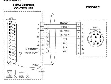
Figure 22 AX4-ENC Encoder Cable Wiring Diagram
