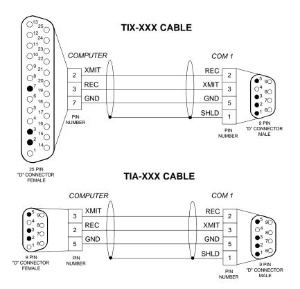
Figure 10 RS232C Serial Communication Cables Wiring Diagram
