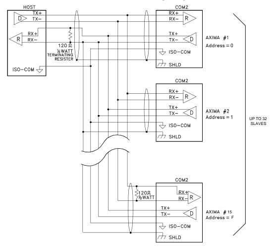
Figure 14 RS485 Four Wire Multi-Drop Wiring Diagram
