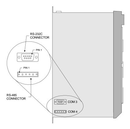
Figure 56 Left-side of AXIMA 2000/4000
