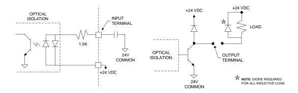
Figure 44 Sinking Inputs and Outputs
