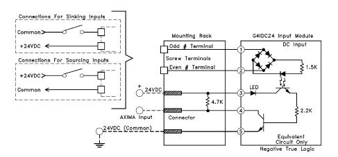
Figure 52 24 VDC Digital Input Module Connection Diagram
