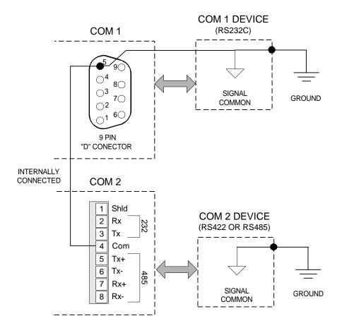
Figure 17 Serial Communications Grounding Diagram
