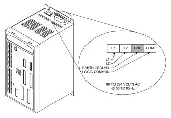
Figure 4 AXIMA 2000/4000 Grounding Point
