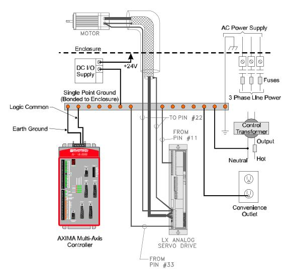
Figure 7 LX Drive and AXIMA System Grounding Diagram
