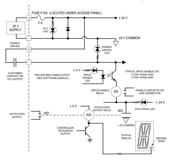
Figure 33 Watchdog, Drive Enable Circuit
