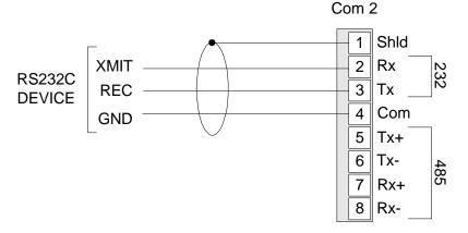
Figure 12 COM 2, RS232C Configuration
