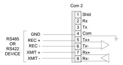
Figure 16 COM 2, RS485 Configuration
