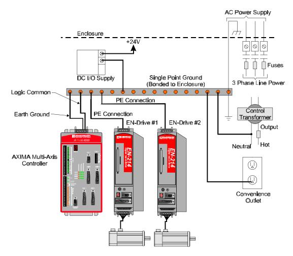
Figure 5 E Series Drive and AXIMA System Grounding Diagram
