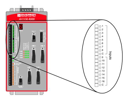
Figure 34 Inputs Location on the Front Panel of the AXIMA 2000/ 4000
