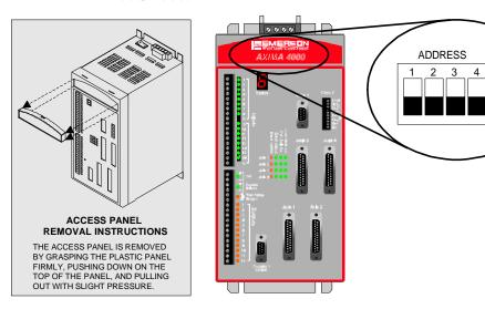
Figure 18 AXIMA 2000/4000 Address DIP Switch Location
