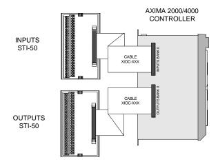
Figure 47 AXIMA 2000/4000 Direct Wiring Option Using STI-50's
