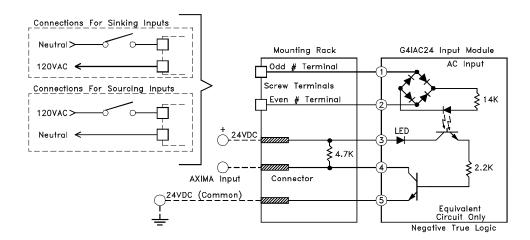
Figure 53 120 VAC Digital Input Module Connection Diagram
