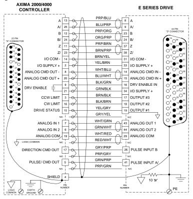
Figure 26 AXIMA 2000/4000 to E Series Drive Connections
