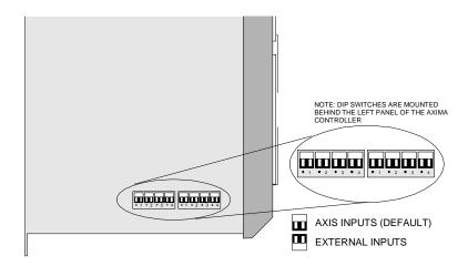
Figure 40 Analog DIP Switch Location Behind the Left-Side Panel of the AXIMA 2000/4000
