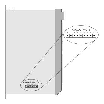
Figure 41 Location of Analog Inputs
