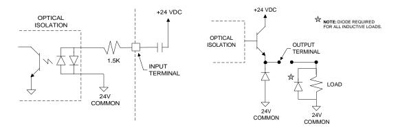
Figure 45 Sourcing Inputs and Outputs
