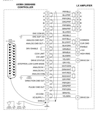
Figure 28 AXIMA 2000/4000 to LX Amplifier Connections Using The AX4-GP Cable (Torque Mode)
