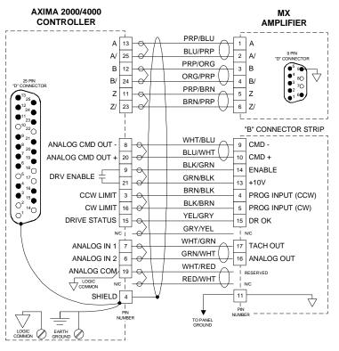
Figure 27 AXIMA 2000/4000 to MX Amplifier Connections Using The AX4-MX cable (Torque Mode)
