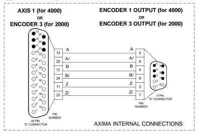
Figure 30 Internal Encoder Connections for AXIMA 2000/4000
