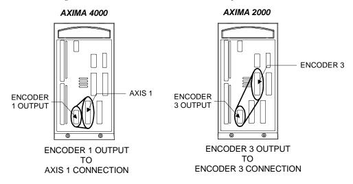
Figure 31 Front Panels of AXIMA 2000/4000 Controllers
