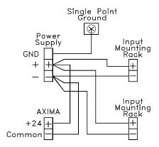
Figure 51 Power Wiring for External L/O Mounting Racks
