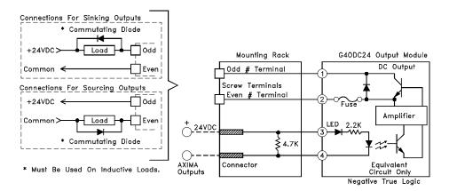
Figure 54 24 VDC Digital Output Module Connection Diagram
