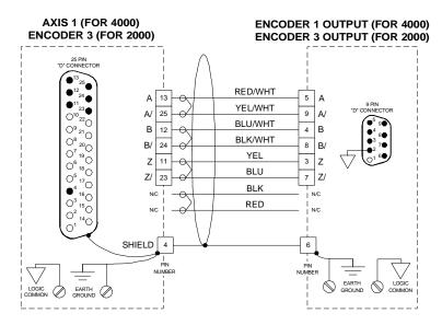
Figure 21 Encoder 1 Signal to another AXIMA Wiring Diagram
