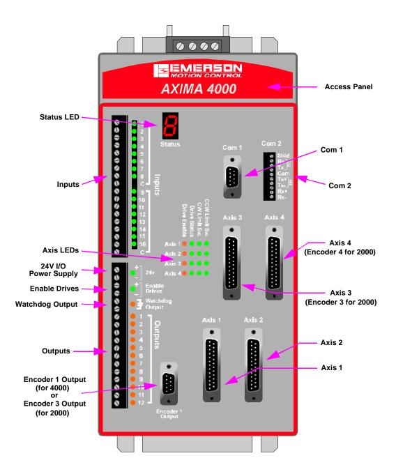
Figure 2 AXIMA 2000/4000 Front Panel Connections
