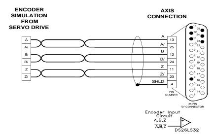
Figure 20 Encoder Simulation Wiring Diagram
