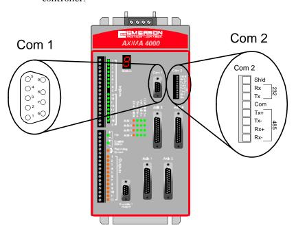
Figure 9 AXIMA 2000/4000 Communication Ports, Com 1 and Com 2
