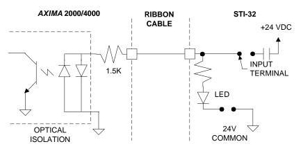
Figure 49 Outputs and Inputs Equivalent Circuit (Sourcing)
