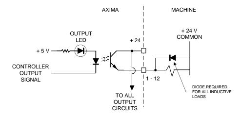
Figure 38 Output Circuit Diagram
