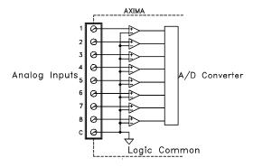
Figure 43 Analog Input Circuit Diagram
