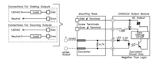
Figure 55 120 VAC Digital Output Module Connection Diagram
