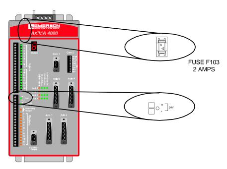
Figure 39 I/O Power Supply Location on the Front Panel of the AXIMA 2000/4000
