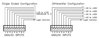
Figure 42 Single Ended Versus Differential Wiring
