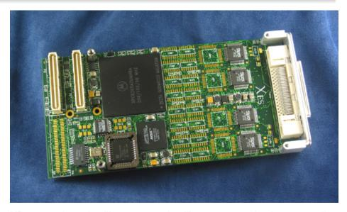
XPort1001 is an intelligent or non-intelligent communications controller targeting low cost, yet high performance applications. XPort1001 combines an array of supported serial protocols, a broad range of serial interface standards, and a flexible I/O routing structure to pack maximum flexibility into an industry standard PMC module.
