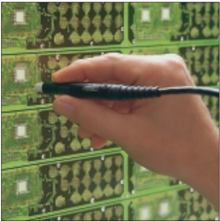
Measurement of the copper thickness in through-holes of printed circuit boards, using the ESL08A probe.
