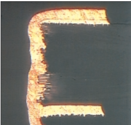
It clearly shows that the voids, which are result of fibers torn by drilling, were subsequently metallized. This effect also makes optical determination of the copper thickness more difficult.
