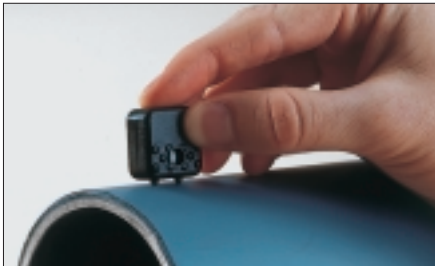
Measurement of synthetic corrosion prevention coatings on pipes using the probe EKB10.
