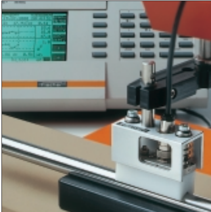
Measurement of the chromium coating on pneumatic cylinders with the probe V2EGA06H mounted in the motorized support stand V12.
