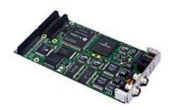
The PMC/860 is a PCI mezzanine card that combines E1 or T1 and TDM telephony bus connectivity with the Motorola
