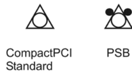
Figure 9: Compatibility Glyphs for CompactPCI Standard and PSB Board Variants
