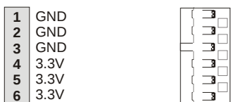
Figure 51: BP4 - PS/2 Power Connector Pinout
